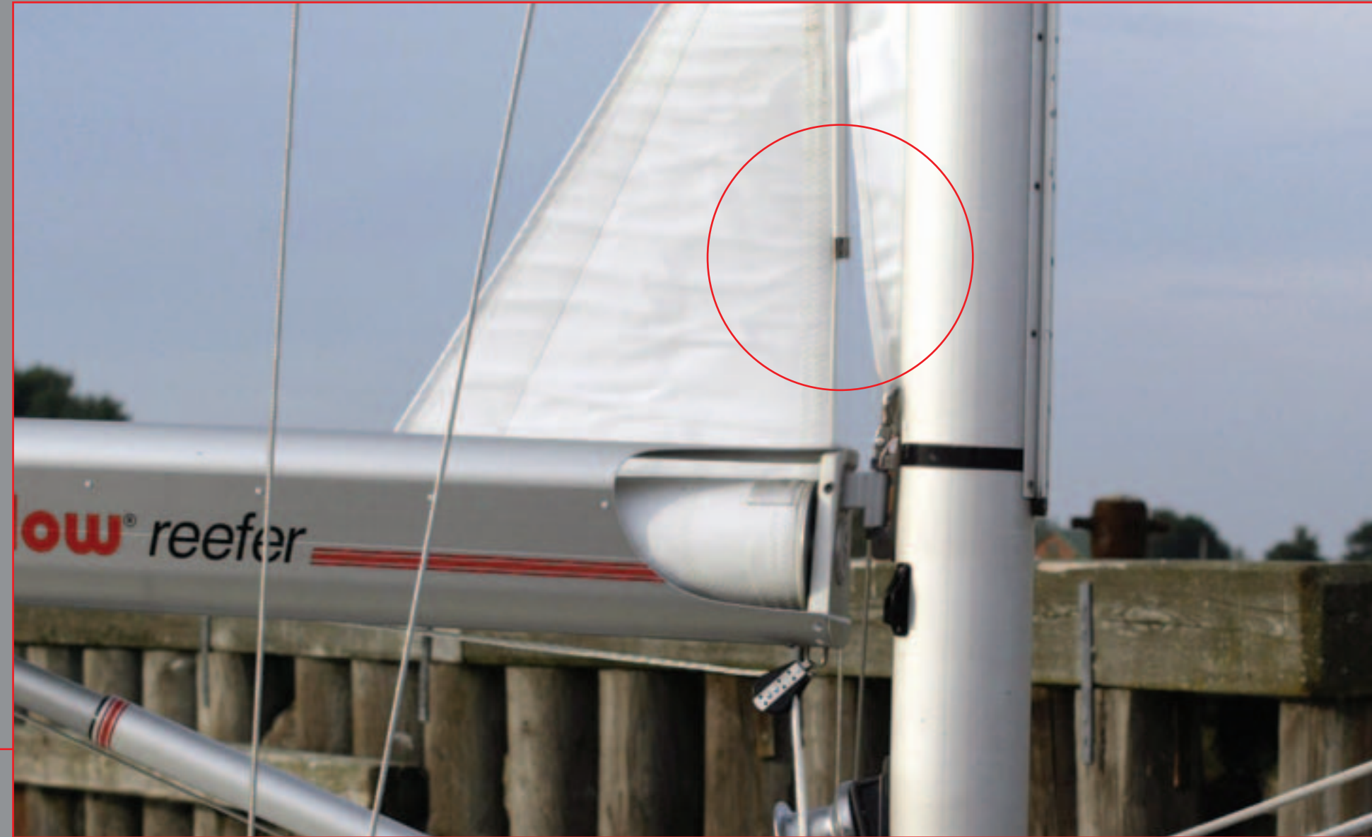
The sail guide will make sure the sail to be taken into the track's groove easy and smoothly. The bottom part of the mast track is flexible constructed so it makes sure the sail to roll down.
