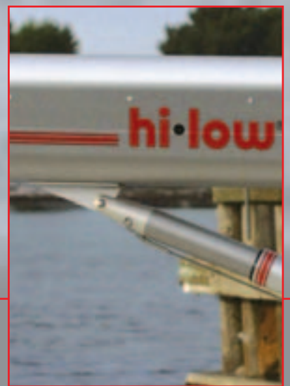
• Boomvang The booms position is very important for the function of the boom. Therefore the built-in gas-spring is lifted to the right angle when the sheet is slacked.
