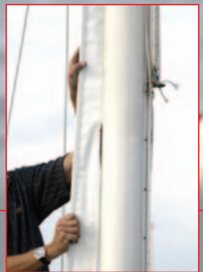
• Sail track The tapered sail track is placed direktly into the mast groove.
