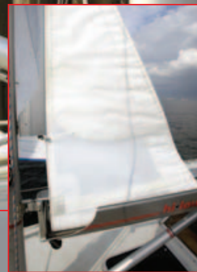
• Hi-low sail The sail has to be special designed for Hi-low reefer and delivered from approved sailmaker.
