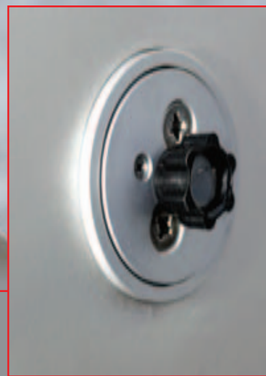
• Outhaul The sail can be stretched by means of adjustment screw at the end of the boom.
