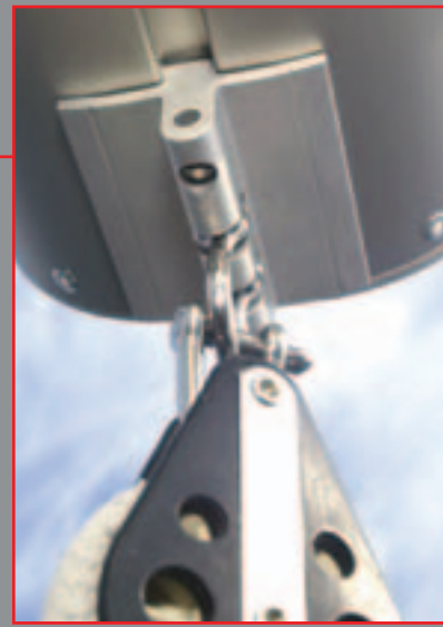
• Adjustable mainsheet bracket Moveable and will be locked with a special screw.
